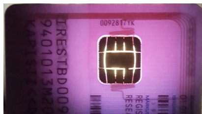
Figure 3.20: A dual-interface chip and antenna in an IDEMIA-powered ID card
