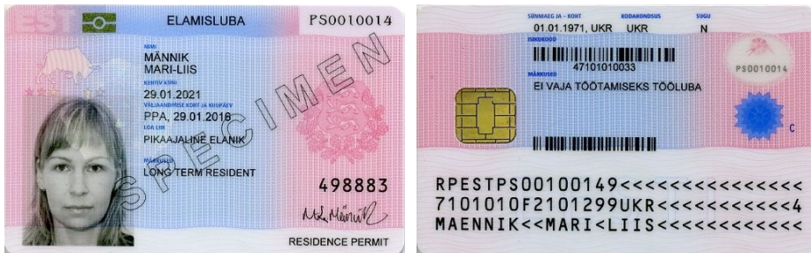
Figure 11: A jTOP SLE66/SLE78-powered residence permit card issued from 2011-01-01 [182]. The 6-digit Card Access Number (CAN) was introduced for the SLE78-powered cards.
