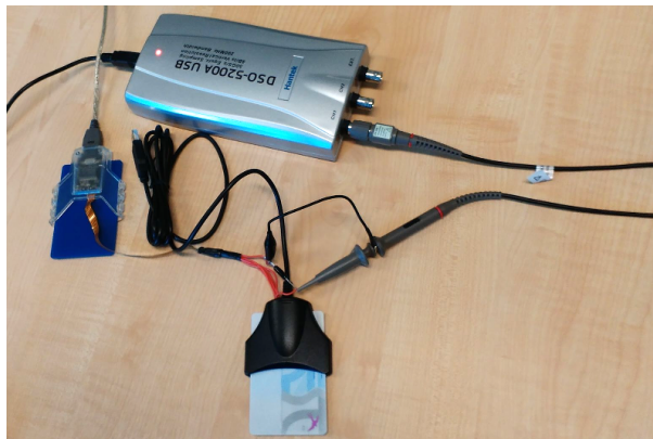
Figure 42: Smart card power consumption analysis setup
