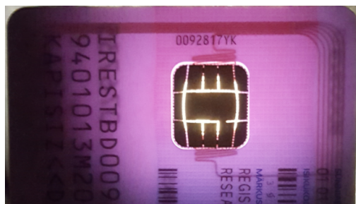
Figure 22: A dual-interface chip and antenna in an IDEMIA-powered ID card
