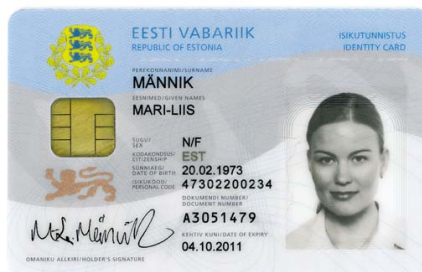
Figure 5: A MICARDO-powered identity card with a squared contact layout designed chip [174]
