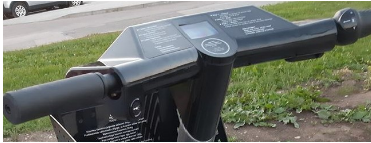
Fig. 5: Smart bike handlebar with built-in NFC card reader (in the center)
